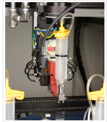
SCS Tower jet valve
