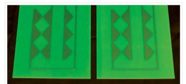
Parylene C-UVF (left) and Parylene C (right) coated boards under visible light.
